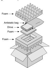
Figure 6. Seagate drive and approved packing materials
