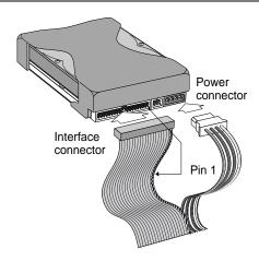
Figure 4. Cable connectors
