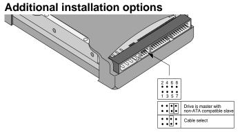
Figure 5. Non-ATA compatible and cable select jumpers
