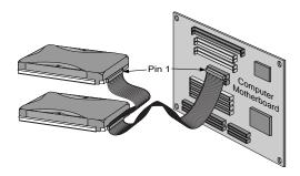
Figure 2. Attaching the cables
