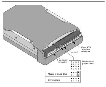
Figure 1. Master and slave jumper settings
